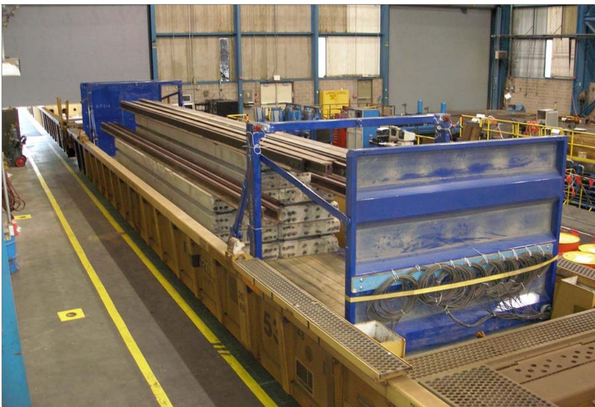
Figure 2. Flat Rack Loaded to Twice its Maximum Capacity (137,000 pounds)
